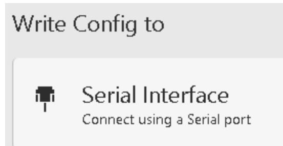
6. Ensure your serial port and baud rate are set correctly
