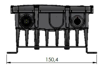
The device physical dimensions and the holes in millimetres with wall mount parts (WP0135).
