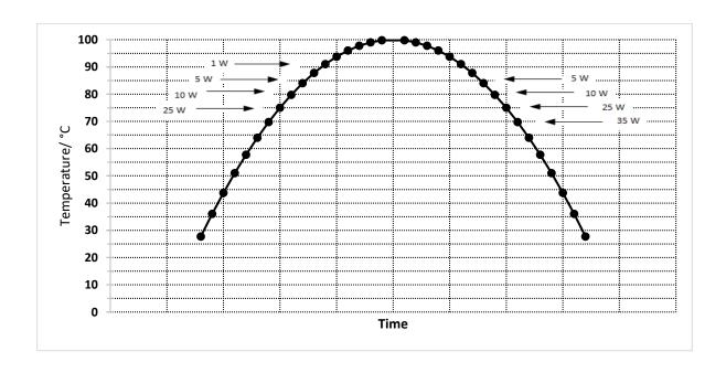
The modem has a built-in self protecting mechanism to prevent an RF power amplifier to overheat. The RF power amplifier temperature is measured and controlled regularly based on data from a temperature sensor on the printed circuit board. Because of the temperature is slowly changing phenomenon, the temperature is measured at the beginning of each transmission and every 10 s period thereafter.
