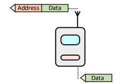
Transmission address has been set OFF. Radio modem will transmit the data packet as such. Transmission addressing has been set ON. The radio modem will add the primary TX address to the beginning of the data packet.
