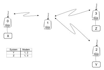
The above figure represents a network containing four (4) radio modems. Each radio modem is given a unique address (0...3). A terminal device has been attached to the three of the four radio modems and they communicate with each other using terminal addresses X, Y and Z, respectively. Radio modem 0 and terminal device X together constitute the base station of the network and all routing information of the network has been programmed into this base station.
