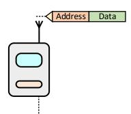
Reception addressing has been set ON and either the primary or secondary RX address of the radio modem is identical to the address of the received data packet.
