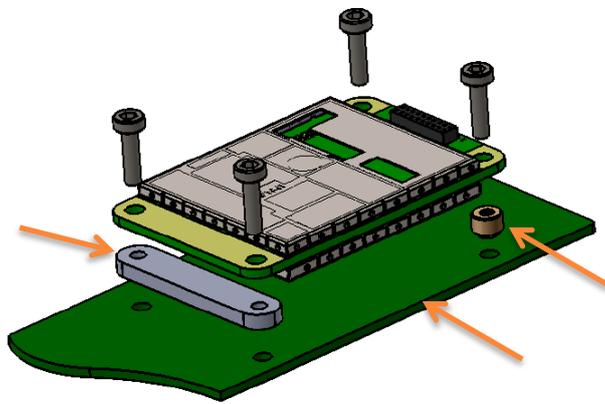
Figure 5.1 Example of module attachment to application PCB.
