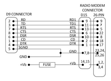
$FUSE = 1 \text{ A slow } (+6 \dots +30 \text{ V assembly}) \text{ or } 2.5 \text{ A slow } (+3 \dots +9 \text{ V assembly})$
