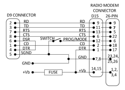
FUSE = 1 A slow ( $+6 \dots +30 \text{ V}$  assembly) or 2.5 A slow ( $+3 \dots +9 \text{ V}$  assembly) SWITCH = Programming mode switch (ON=Programming mode, OFF=Data transfer mode)
