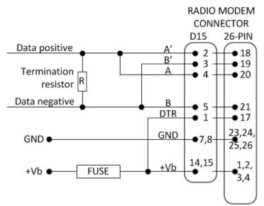
FUSE = 1 A slow ( $+6 \dots +30 \text{ V}$  assembly) or 2.5 A slow ( $+3 \dots +9 \text{ V}$  assembly)
