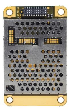
SATELLINE-M3-R4 is a flexible module which makes it a suitable unit for different uses. It is an updated version of M3-R3 module. It has two modulations more; 8FSK and 16FSK which gives more speed to the radio interface.
