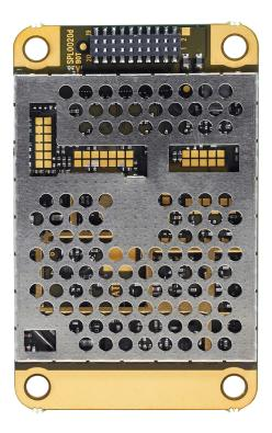
SATELLINE-M3-TR4 is a flexible module which makes it a suitable unit for different uses. It is an updated version of M3-TR3 module. It has two modulations more; 8FSK and 16FSK which gives more speed to the radio interface.
