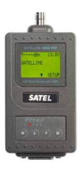
The SATELLINE-3AS VHF operates on the 135...174 or 218...238 MHz frequency bands. The radio modem is compatible with the most widely used serial interfaces RS-232, RS-485 and RS-422. The SATELLINE-3AS(d) VHF with 5 W output power and a heat sink is the appropriate choice when continuous transmission (when transmitter duty cycle exceeds 20%) is required. In mobile fleet management applications, use of VHF frequencies reduces signal fading significantly.
