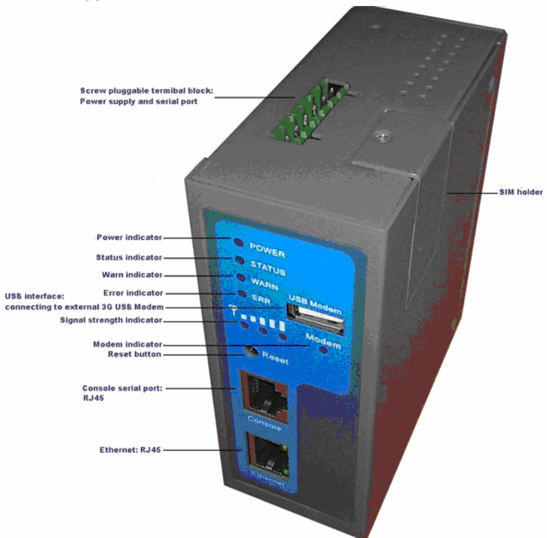
Figure 2.2 Front Panel (USB host type – without built in cellular module)
